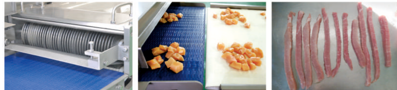
Easy-to-change blade assemble ensures the production convenience.
